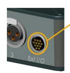
MIXY also routes the analogue output to the 12pin Minicon with independent level control, primarily for use with radio TXs. Select "RF" and adjust MOL between -40dB and 14dBu.
