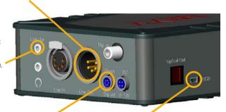
Iso outputs of Ch1, 2 § 3 are available as unbalanced outputs at MIXY'S HR10-6 connector.
