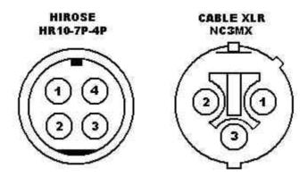
All connectors viewed from soldering side. The pin numbers indicate the standard set by MICRON and all cables in this manual.
